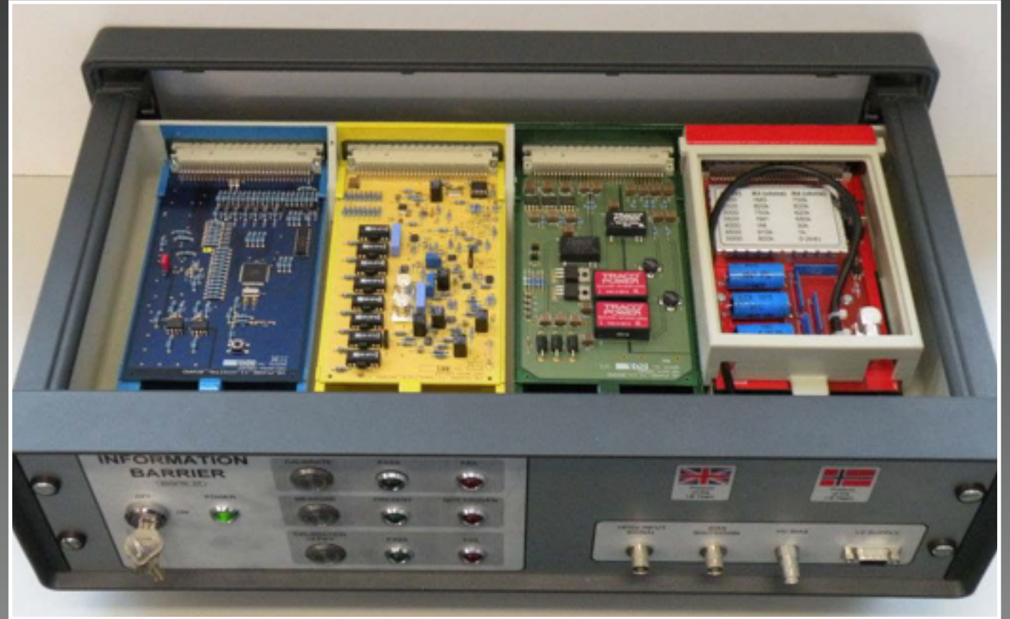
2nd Prototype of the Information Barrier developed as part of the UK-Norway Initiative
