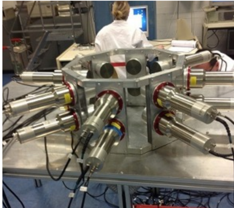
Liquid scintillator passive well counter to determine the plutonium mass in samples of unknown size
