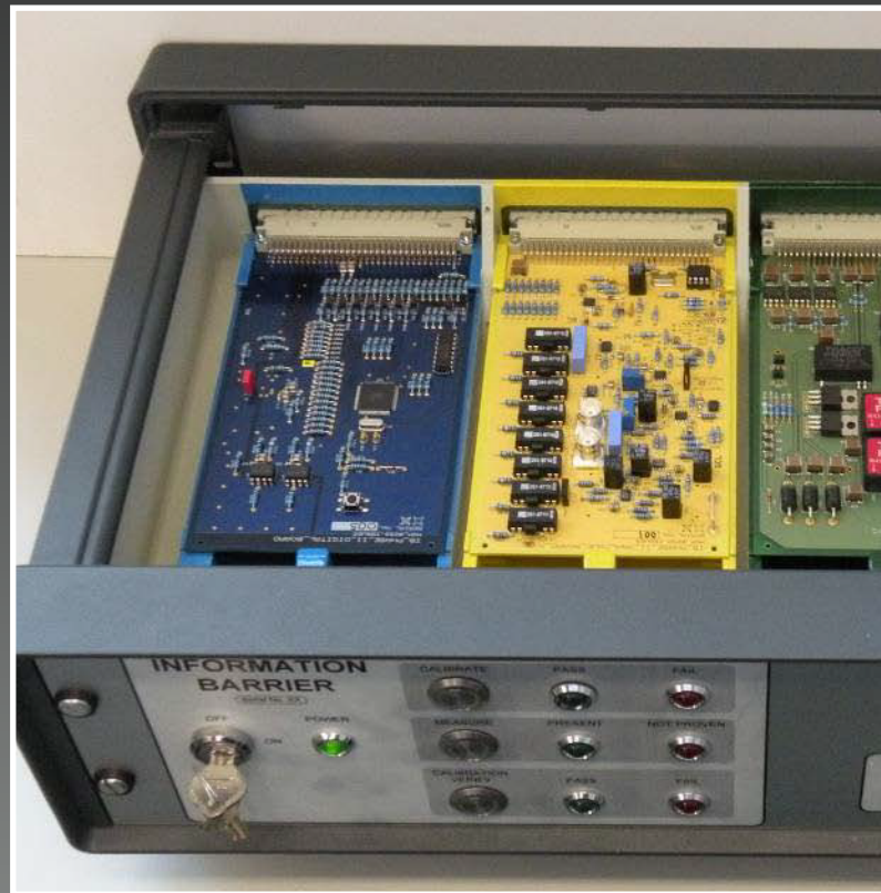
2nd Prototype of the Information Barrier developed as part of the UK-Norway Initiative Source: Ole Reistad et al.
