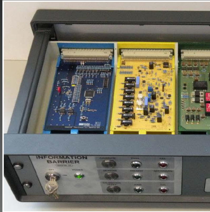
2nd Prototype of the Information Barrier developed as part of the UK-Norway Initiative Source: ukni.info
