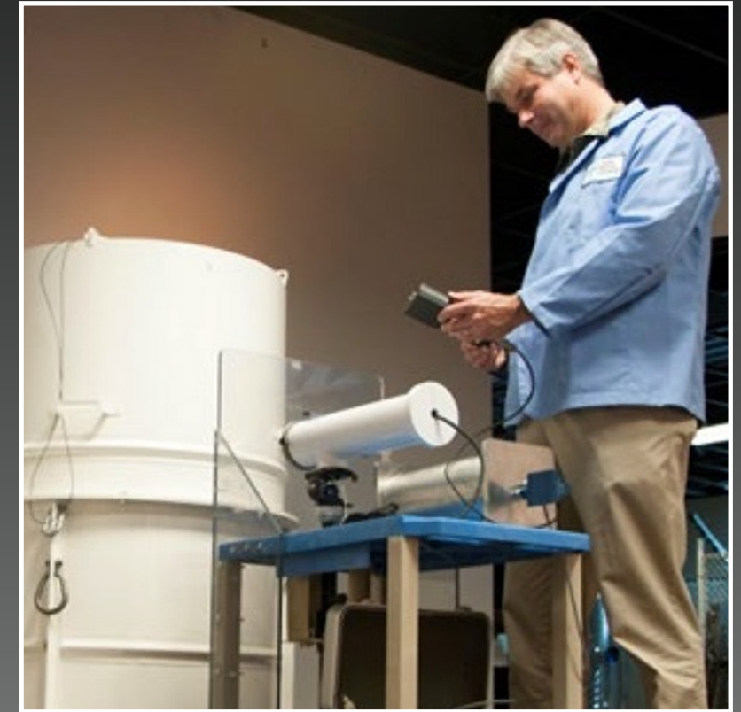
Trusted Radiation Identification System (TRIS) developed by Sandia National Laboratories Source: U.S. Department of Energy
