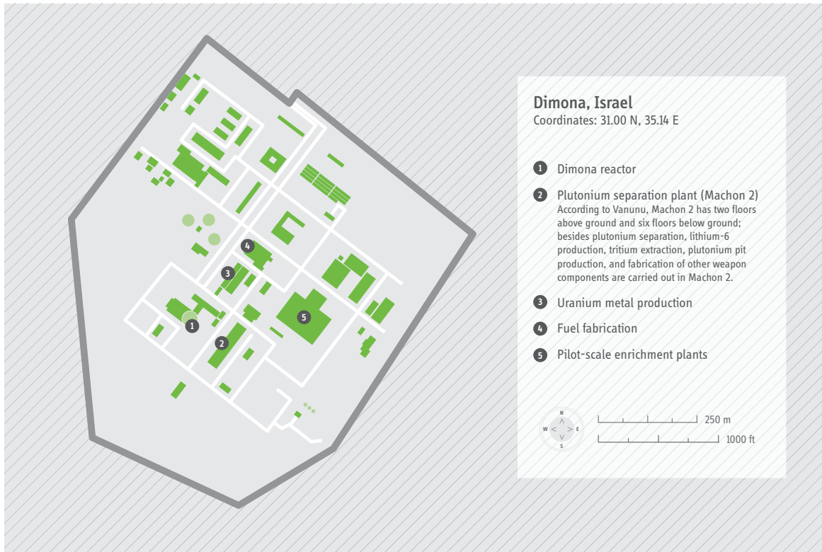
Figure 1: Map of the Dimona site and reported designations and purposes of separate units. Based on drawings published in a 1961 U.S. government memo and in a 1989 book on the arms race in the Middle East.
