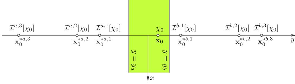
FIG. 7. Images of an elastic multipole with the Airy stress function  $\chi_0$  at position  $\mathbf{x}_0$  between the two parallel traction-free edges at  $y = y_a$  and  $y = y_b$ . See text for the detailed description.
