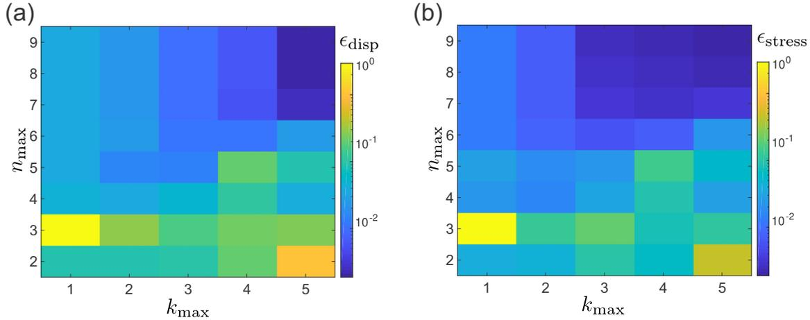
FIG. 10. The normalized errors for (a) displacements  $\epsilon_{\text{disp}}(n_{\text{max}}, k_{\text{max}})$  and (b) stresses  $\epsilon_{\text{stress}}(n_{\text{max}}, k_{\text{max}})$  as defined in Eq. (27) for the deformation of an elastic strip with a single hole [see Fig. 8(a)].
