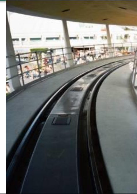
Active element of LIM in guideway
