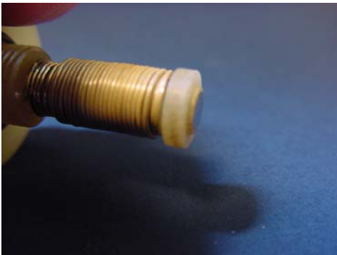
Image 2. Side view of electrode assembly. The Pt/Ir electrode elevated over flat surface and that after putting gas permeable membrane protect biological sample against leakage.
