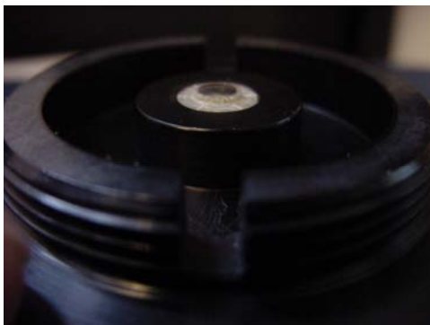
Image 1. View of micro-cell body with inserted electrode assembly that is ready for filling by electrolyte (0.1 M KCl) and covering by gas permeable membrane ( \sim 1 \mu\text{m} thickness).
