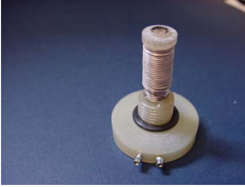
Image 2. View of electrode assembly with polished Pt/Ir electrode and wrapped silver wire.
