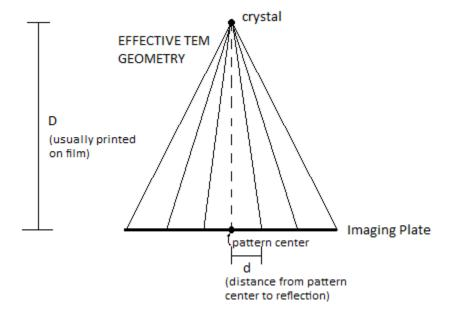
For an electron energy E in KeV, D and d in the same units, and  $n=\sqrt{h^2+k^2+l^2}$ , the d-spacing of the reflection is given by:
