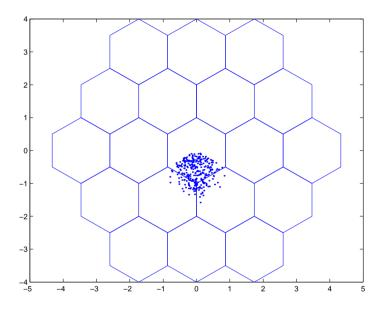
3GPP Uplink Evaluation Tool: 19 cells in three hexagons
