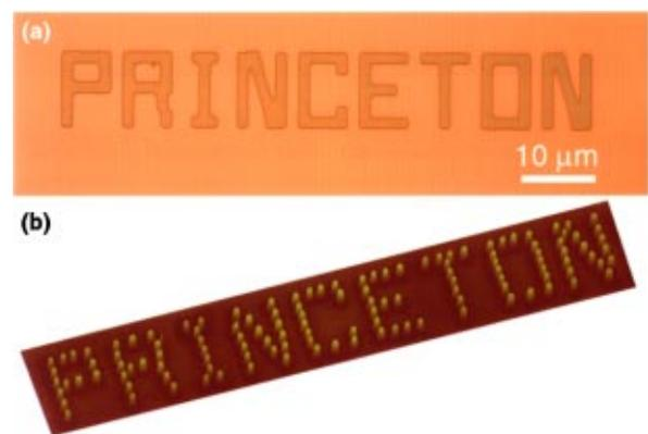
FIG. 6. (a) Optical micrograph of a protruding line pattern of the word “PRINCETON” on the mask and (b) AFM image of LISA of PMMA pillars that formed under the mask pattern.
