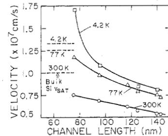
Fig. 3. Calculated average electron velocities of the devices with different electrical channel lengths at 300, 77, and 4.2 K.
