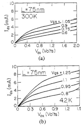
Fig. 1.  $I$ - $V$  characteristics of a 75-nm-channel MOSFET (a) at 300 K and (b) at 4.2 K.
