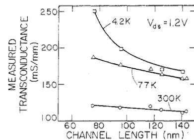
Fig. 2. Measured transconductances of the devices with different electrical channel lengths at 300, 77, and 4.2 K.
