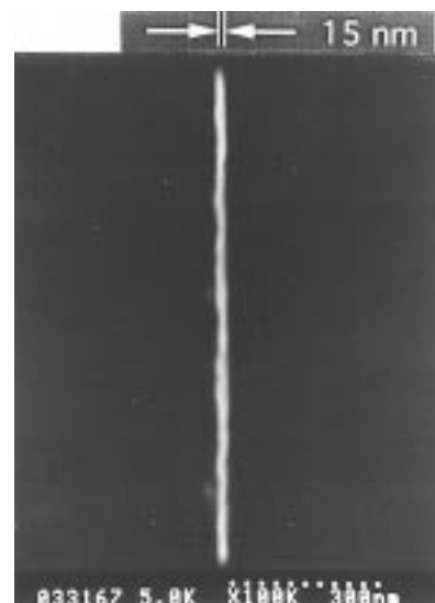
Fig. 2. SEM image of an isolated Ni bar that is 15-nm wide, 1- \mu m long, and 35-nm thick.
