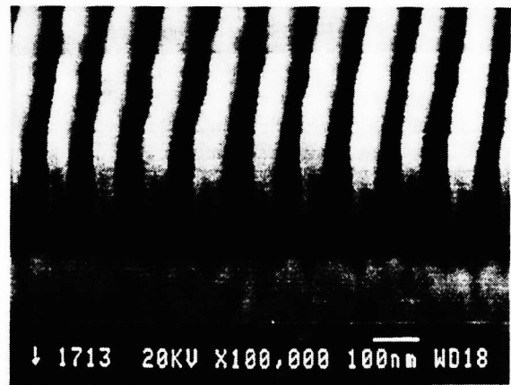
Fig. 2. Amorphous silicon gratings with 100 nm period and 240 nm thickness on silica.
