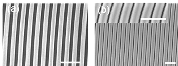
FIG. 1. (a) Top view scanning electron microscopy (SEM) image of nanofluidic channels with a trench width of 85 nm. The dark area is the trench. (b) The channels were narrowed down to less than 20 nm by controlled *e*-beam deposition. The inset shows the channel width at a higher magnification. The scale bars are all 500 nm.
