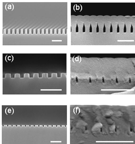
FIG. 3. (a), (b) Nanofluidic channels with trench width of 85 nm were sealed by a single step SiO<sub>2</sub> sputtering, the sealed channel was reduced to nearly 55 nm after the sealing process. The experiment was repeated (c), (d) for 65 nm channels which were reduced to less than 17 nm after sealing. And (e), (f) for 55 nm wide channels which were reduced to less than 10 nm width. The scale bars are all 500 nm.
