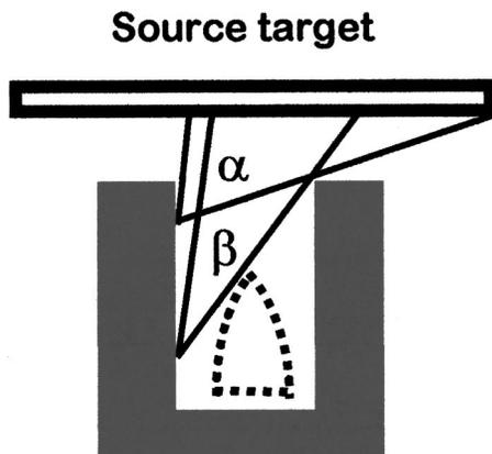
FIG. 2. A schematic illustration of the sputtering deposition process.
