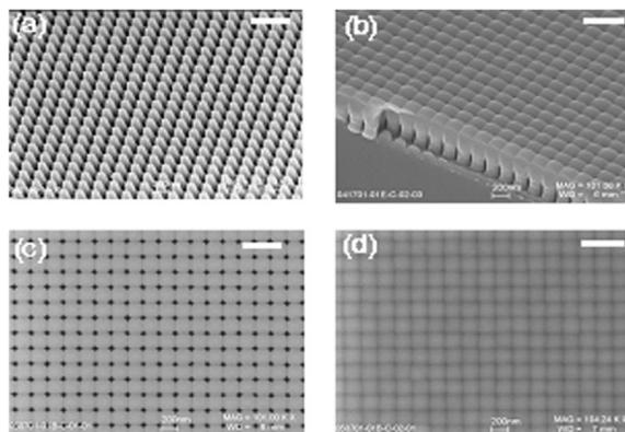
FIG. 4. (a), (b) Nanofluidic pillar array structures before and after sealing by the sputtering process. (c), (d) Top view images of half-sealed pillar array structures with 200 nm of SiO<sub>2</sub> deposited and a completely sealed structure after 400 nm of SiO<sub>2</sub> was deposited. The scale bars are all 500 nm.
