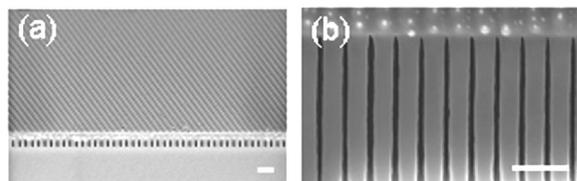
FIG. 5. (a) SEM image shows the “roof” and profile of the nanochannels sealed by the  $\text{SiO}_2$  sputtering process. (b) Buried nanochannels under the sealing roof were shown to be perfectly intact after sealing. The scale bars are all 500 nm.
