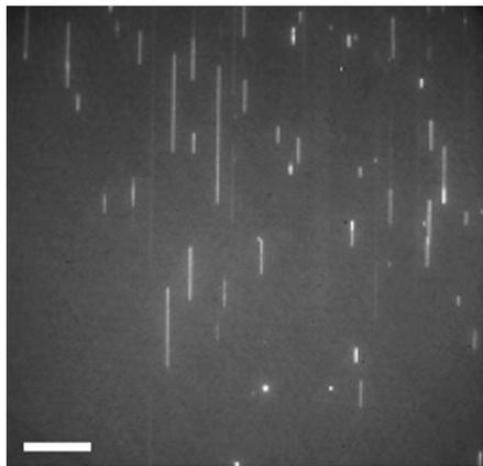
FIG. 6. CCD image of  $\lambda$ -phage DNA concatemers stretched in nanofluidic channels. The scale bar is 30  $\mu\text{m}$ .
