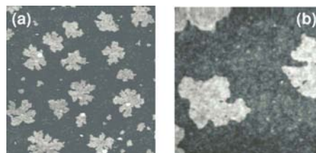
FIG. 1. Atomic-force micrographs of SAM formed on unpatterned SiO 2 for 5 min. Scales: (a) x=y=2.5\ \mu\text{m} , z=5\ \text{nm} full scale; (b) x=y=750\ \text{nm} , z=5\ \text{nm} full scale.
