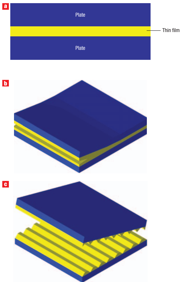
Figure 1 Schematic of the FIS process. a–c , The process comprises the following steps. A thin glassy featureless film (yellow) is confined between two rigid plates (blue) ( a ), the two plates are prised apart from an edge, causing fracture of the film ( b ), and as the fracturing propagates from one edge of the plate to the other edge, the film self-breaks into two complementary sets of gratings of the same period but with nonsymmetrical shapes, one set on each plate ( c ).
