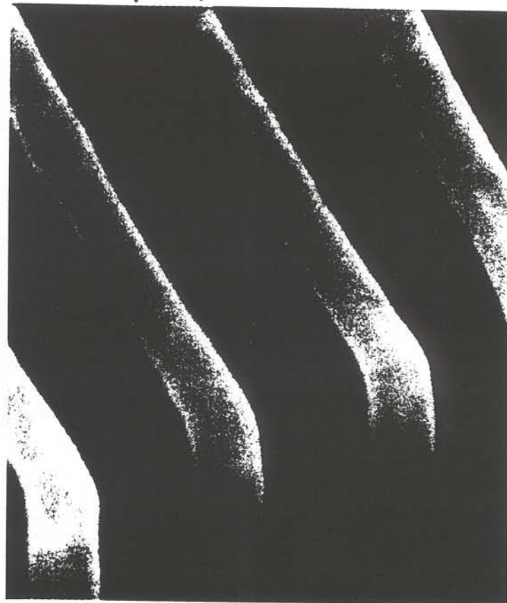
Figure 4: SEM image of a profile of strips formed into a PMMA film by the imprint technique. The strips are 70 nm wide and 200 nm tall, have a high aspect ratio, a surface roughness of less than 3 nm, and nearly perfect 90 degree corners.
