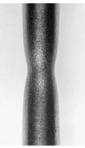
Even at this stage, the material does not suddenly fail: it continues to stretch to the point marked X before breaking. If the load is removed before breaking, the elastic strain is recovered and the metal contracts along the dotted line to point 4. It is the toughness of steel - its resistance to sudden catastrophic failure - that makes it so useful.
