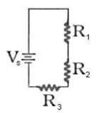
$$\begin{split} R_{Total} &= R_1 + R_2 + R_3 \\ Current, \ I, \ is \ the \ same \ through \ each \ resistor, \ and \\ equal \ to: \ I = V_{Source}/R_{Total} \end{split}$$
