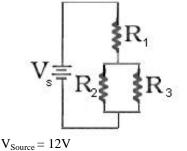
$R_1 = 1000\Omega$   $R_2 = 400\Omega$   $R_3 = 400\Omega$
