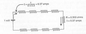
$$I = \frac{V}{R_1 + R_2 + R_3 + R_4 + R_5 + R_6 + R_7 + R_8 + R_9} = \frac{1}{9 \times 0.303} = 0.37 \text{ amps}$$
