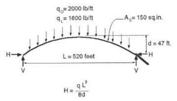
Model for equilibrium of uniform load on each of the four steel arches that make up the central span. Arch is assumed to be three hinged.
