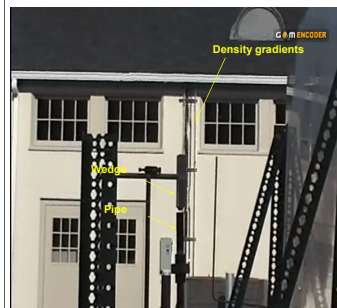
Test conditions: 4" pipe length, 1/2" wedge, burst pressure 1715 psig. Refraction of light due to density gradients indicates sustained burning after spontaneous ignition event.
