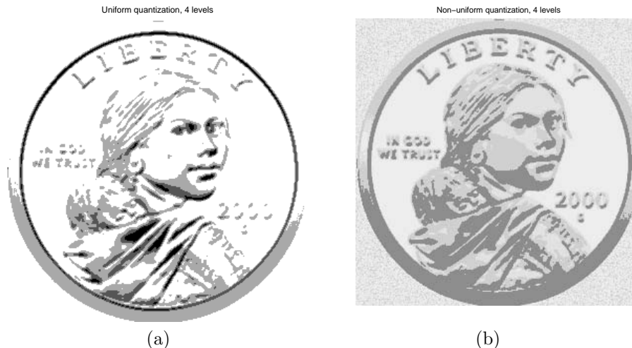
Figure 5.16: (a) Uniformly quantized image. (b) Non-uniformly quantized image
