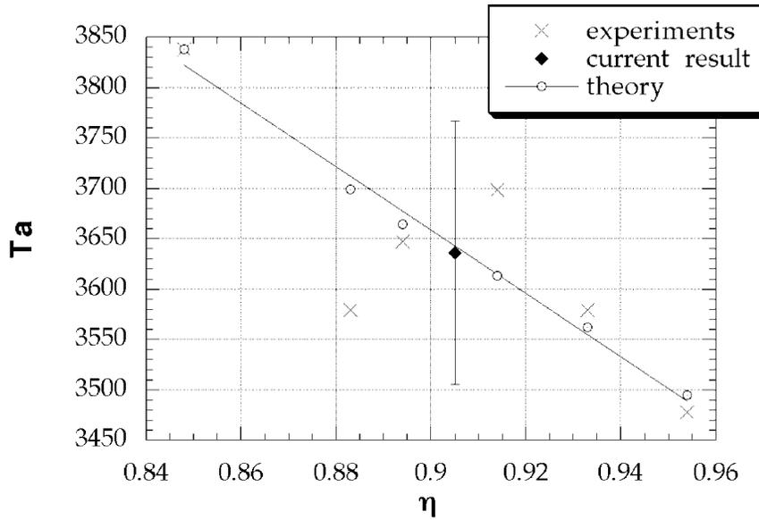
FIGURE 3. Critical values of the Taylor number in ordinary Taylor-Couette flow ( $Re = 0$ ),  $Ta_{c,0}$  as a function of the radius ratio,  $\eta$ .  $\diamond$ , present results. The other experimental ( $\times$ ) and theoretical ( $\circ$ ) values are taken from Lueptow *et al.* (1992) and Cole (1976), and their cited sources. The theoretical values are shown with their best linear curve fit.
