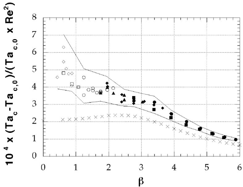
FIGURE 5. Enhanced stability due to axial motion of the inner cylinder normalized by  $Re^2$  as a function of the oscillation parameter  $\beta$ . Symbols are as given in Figure 4. The range of uncertainty in the measurements is given by the distance between the solid lines. The analytical results by Hu & Kelly (1995) for  $Re = 30$  and  $\beta \leq 6$  are indicated by the  $\times$  symbol..
