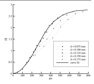
**Figure 2.** Results of Shaw (1960) for different diameter tappings in a 2 inch diameter pipe. Shaw's 'universal' curve is shown as a solid curve. Other curves are for guidance only.
