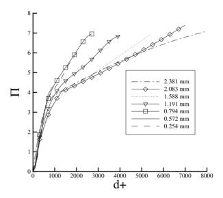
**Figure 7.** Variation of non-dimensional pressure error,  $\Pi$ , with tapping diameter.
