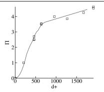
**Figure 5.** Distribution of non-dimensional pressure error data,  $\Pi$  ( $\Box$ ), around curve fit (——),  $Re_D = 3 \times 10^6$ .
