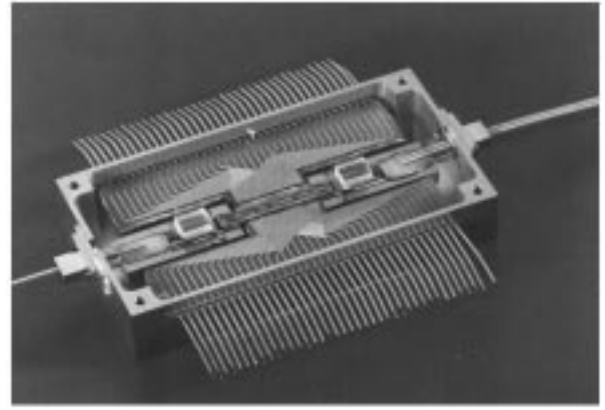
Fig. 11. Packaged 4 \times 4 DOS InP switch matrix.
