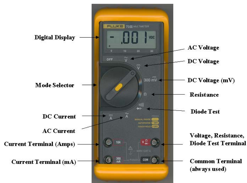
Figure 2.3.3. Fluke handheld multimeter.
