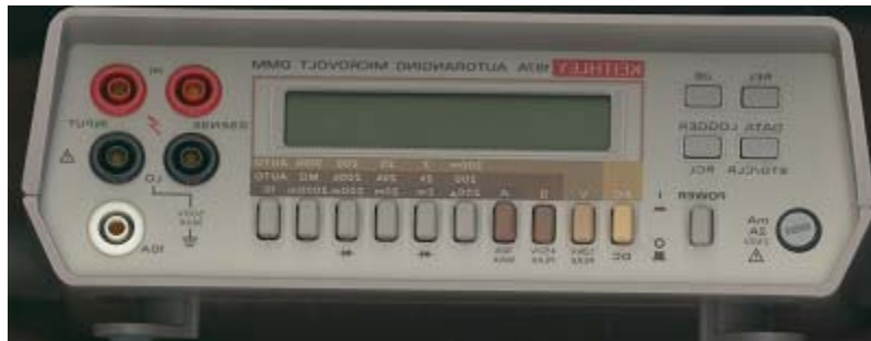
Figure 2.3.4. Keithley tabletop multimeter.
