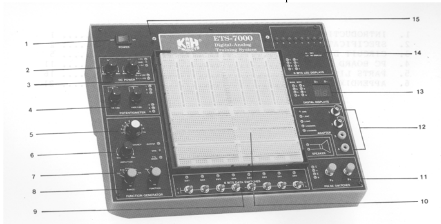
Figure 2.3.1: ETS-7000 Training and Prototyping Board (the trainer ).
