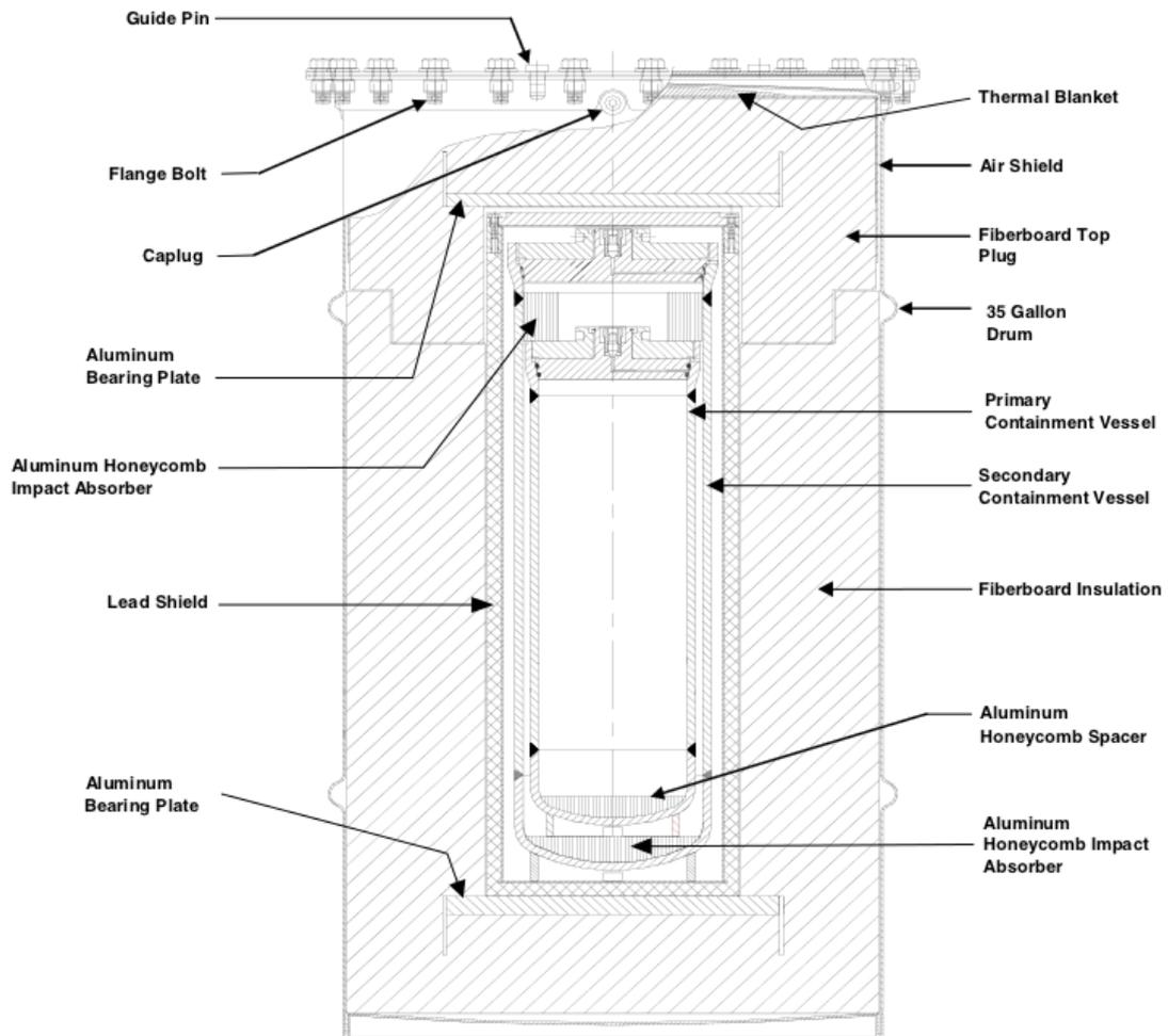
Figure 1: Sketch of 9975 container from [9]. The fiberboard insulation consists of Celotex. The Celotex component is 11.9 cm thick, the overall container has a diameter of 46.4 cm.
