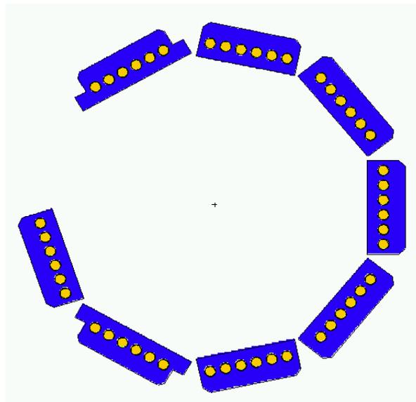
Figure 2 Cross-sectional sketch of the He-3 slab detector from the top. Polyethylene is depicted in blue; the He-3 tubes are marked yellow. The tubes have a length of 35.8 cm, items with a diameter less than 35.8 cm can be placed in the detector.
