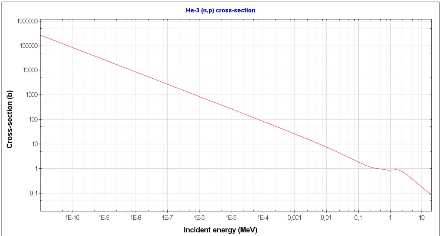
Figure 4: Cross-section of (n,p) reaction in He-3 from ENDF/B-VII.0
