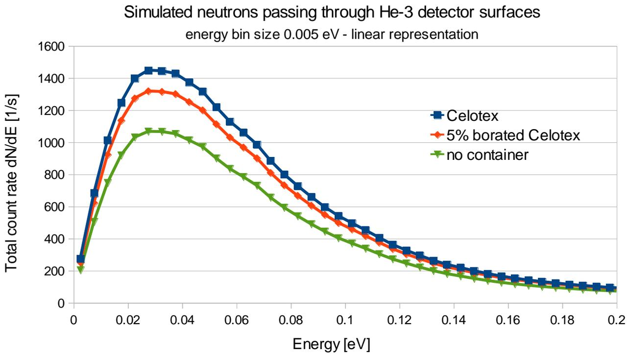
Figure 3: Energy spectrum of the low-energy neutrons (MCNPX PoliMi simulations) entering the He-3 tubes
