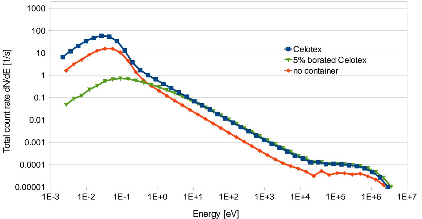
Figure 5: Logarithmic energy spectrum of all neutron (MCNPX PoliMi simulations) reflected back into fissile material for the different container configurations
