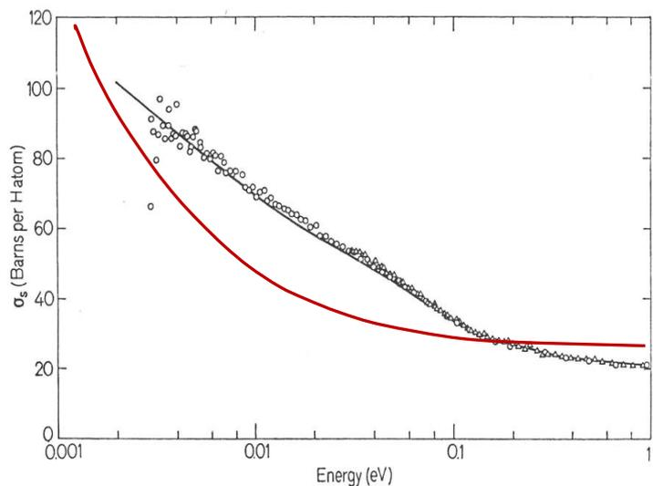
Figure 3: The derived (black line) and measured (dots) total thermal polyethylene cross-section is shown, taken from *D. Sprevak and J.U. Koppel, Neutron Scattering by Polyethylene, Nukleonik 12, 1969*. The red line represents the total nuclear cross-section.
