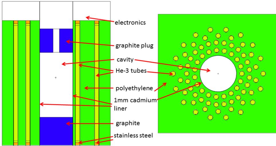
Figure 1: Model of the Passive Scrap Multiplicity Counter. White indicates air or materials of little relevance for neutron transport, blue indicates graphite, orange indicates stainless steel, the shiny green indicates polyethylene, the greenish yellow indicates He-3. The total size of the detector is 661 x 661 x 942 mm (length x width x height).
