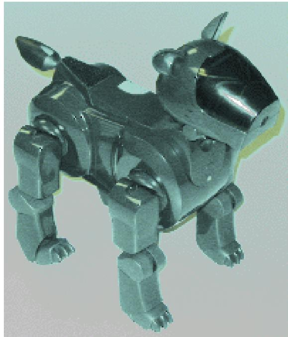
Figure 1: The Sony AIBO entertainment robot, model ERS-210.
