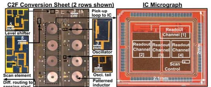
Fig. 7: Photograph of prototype, including 130nm CMOS IC and C2F sheet based on a-Si TFTs fabricated in house on  $50\mu m$  polyimide.
