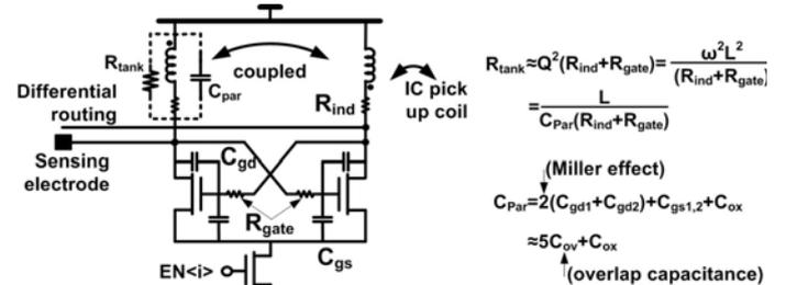
Fig. 3: Thin-film LC sensing oscillator circuit and oscillation condition derivation.
