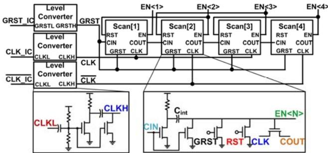
Fig. 5: TFT level-shifters and scan circuits.
