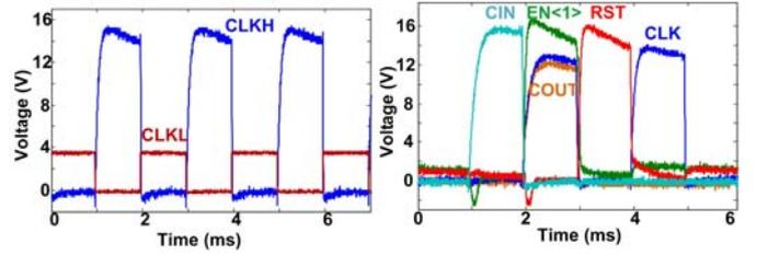
Fig. 6: Operation waveform of level converter and scan element.
