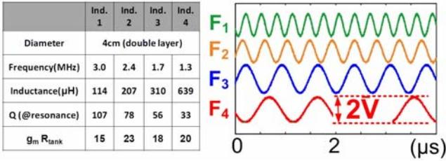
Fig. 4: Flexible planar inductor parameters and four channel SO waveforms with minimal frequency separation of 400kHz.
