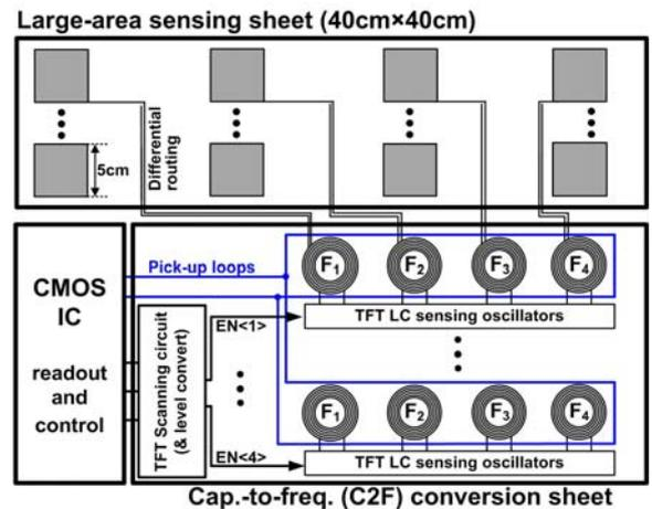
Fig. 1: Architecture of 3D pixel-based capacitance-sensing system.
