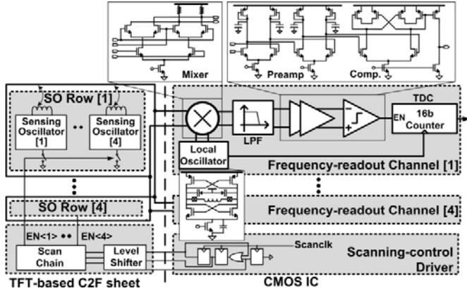
Fig. 2: C2F sheet and CMOS IC details.
