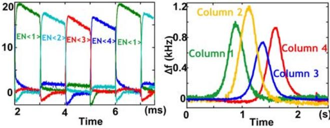
Fig. 9: Measured waveforms of scanning circuit output and readout output with a hand swiping 6cm above a row of electrodes.
