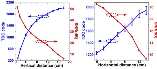
Fig. 8: Measured TDC output and SNR versus vertical distance and horizontal displacement of a hand with respect to sensing electrode.
