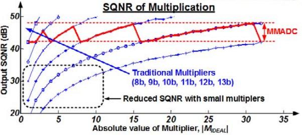
Figure 18.4.3: MMADC results in multiplier quantization error that scales with  $2^{M_d}$  (and thus  $M_{QUANT}$ ), giving relatively constant output SQNR over arbitrarily large range of multipliers.
