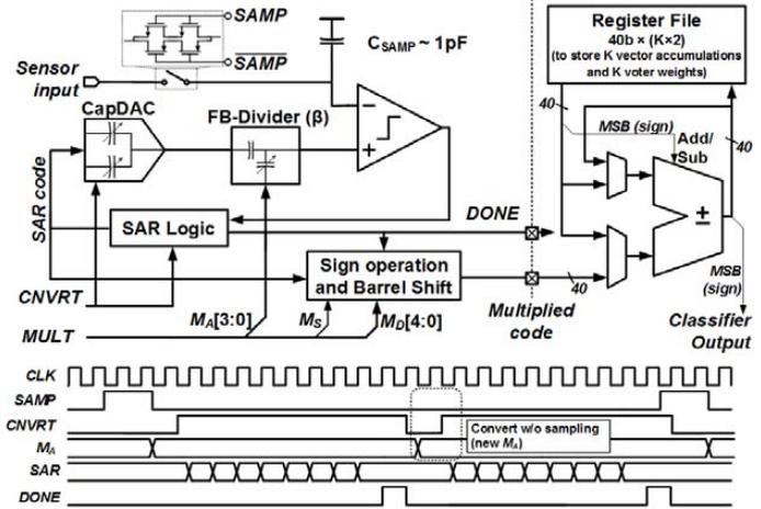
Figure 18.4.2: MMADC implements mixed analog/digital multiplication, with analog multiplication via feedback attenuation by FB-Divider and digital multiplication via barrel shifting.
