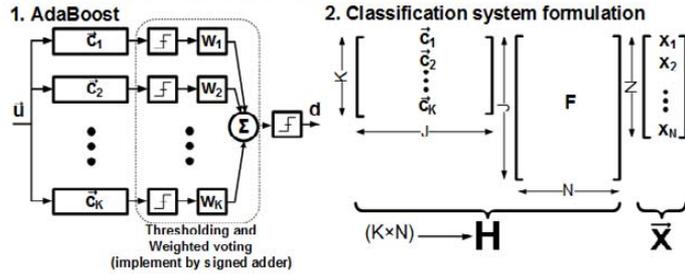
Figure 18.4.1: Compared to conventional system (top), AdaBoost enables ensemble of K linear classifier vectors  $\tilde{c}_i$  which can be combined with linear feature extraction F in the matrix H.
