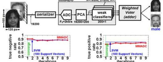
Figure 18.4.5: Two MMADC systems achieve classification performance near that of an SVM with  $\sim 9.7\times$  and  $\sim 23\times$  energy reduction vs. conventional systems (assuming 3.8pJ for 13b digital multiplication and 0.95pJ for 40b digital addition in 130nm CMOS).
