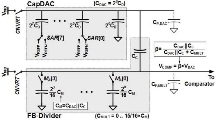
Figure 18.4.4: SAR feedback path, composed of CapDAC and FB-divider, wherein FB-Divider applies switchable attenuation factor  $\beta$  through capacitive division implemented with  $C_{MULT}$ .
