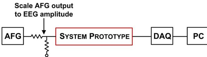
Fig. 18. Setup for compressively sensed EEG acquisition.
