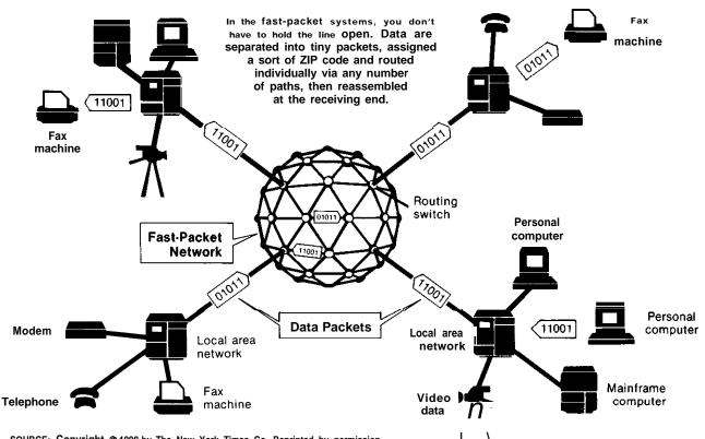
Figure 3-3—Fast-Packet Switching (Hello Central)
