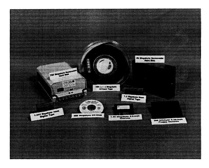
A common form of hardware incompatibility is that of the media used to store data. The picture shows a frustrated user's exhibit of the many media on which he received remotely sensed Earth data during Operation Desert Storm. Source: United States Army Topographic Engineering Center.
