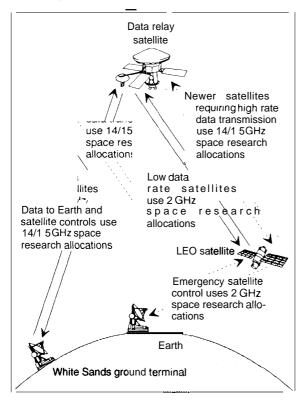
Figure 2-1 I-Data Relay Satellite System
