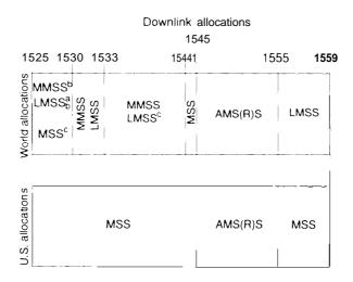
Figure 2-5-WARC-92 L-Band Mobile-Satellite Service Allocations
