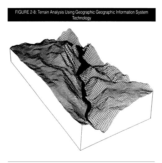
The U S Geological Survey prepared this dlgltal elevation model of the Hetch Hetchy Canyon in Yosemlfe National Park, California using aerial photographs
