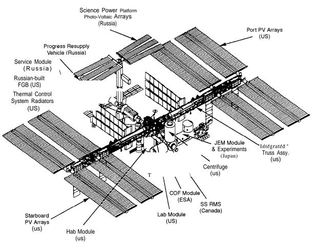
FIGURE 3-4: Schematic Drawing of the International Space Station
