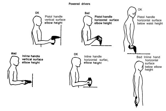
Figure 7-8.—Good and Bad Designs for Powered Drivers
