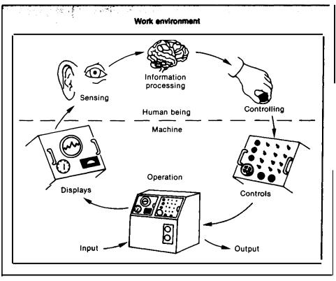
Figure 7-1.—Schematic Representation of a Human-Machine System
