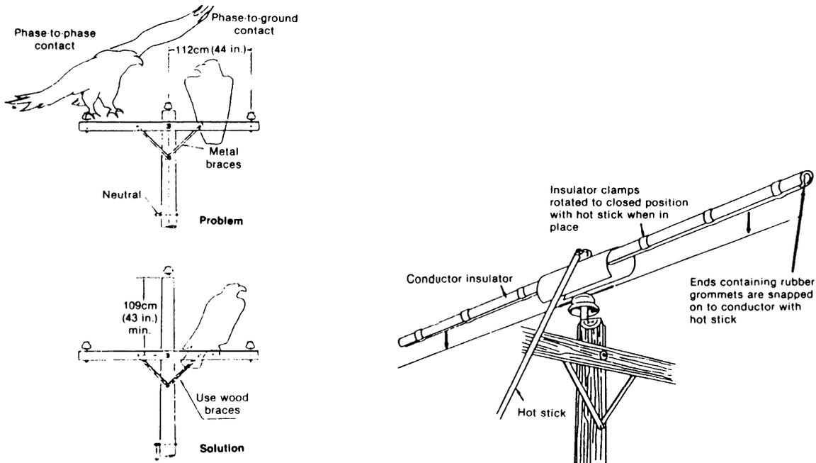
Vertical separation of the center and two outside conductors precludes the electrocution hazard on one type of pole
