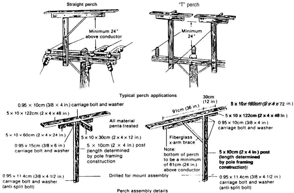
Artificial perches mounted above existing poles as an alternative to Pole modification (suitable primarily for treeless areas) and perch assembly details.
