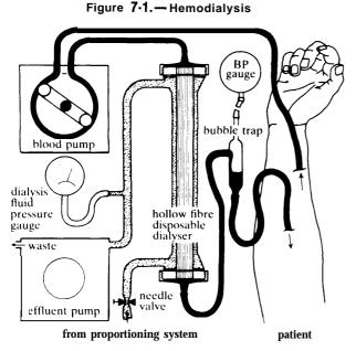
Blood is taken from the arterial tube and pumped through the hollow-fiber disposable dialyzer before returning through an air trap to the patient. Dialysis fluid flows in the opposite direction from a proportionating system, which makes it from water and concentrate. A number of safety devices (not shown) monitor the temperature, flow, and pressure of the dialysis fluid and the presence of air bubbles in the blood stream.
