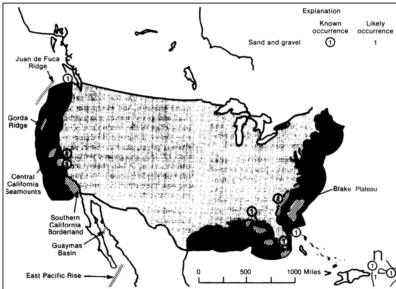
Significant sand and gravel deposits lie on the continental shelf near urban coastal areas. As local onshore supplies of construction aggregate become exhausted, offshore deposits become more attractive. Sand is also needed for beach replenishment and erosion control.
