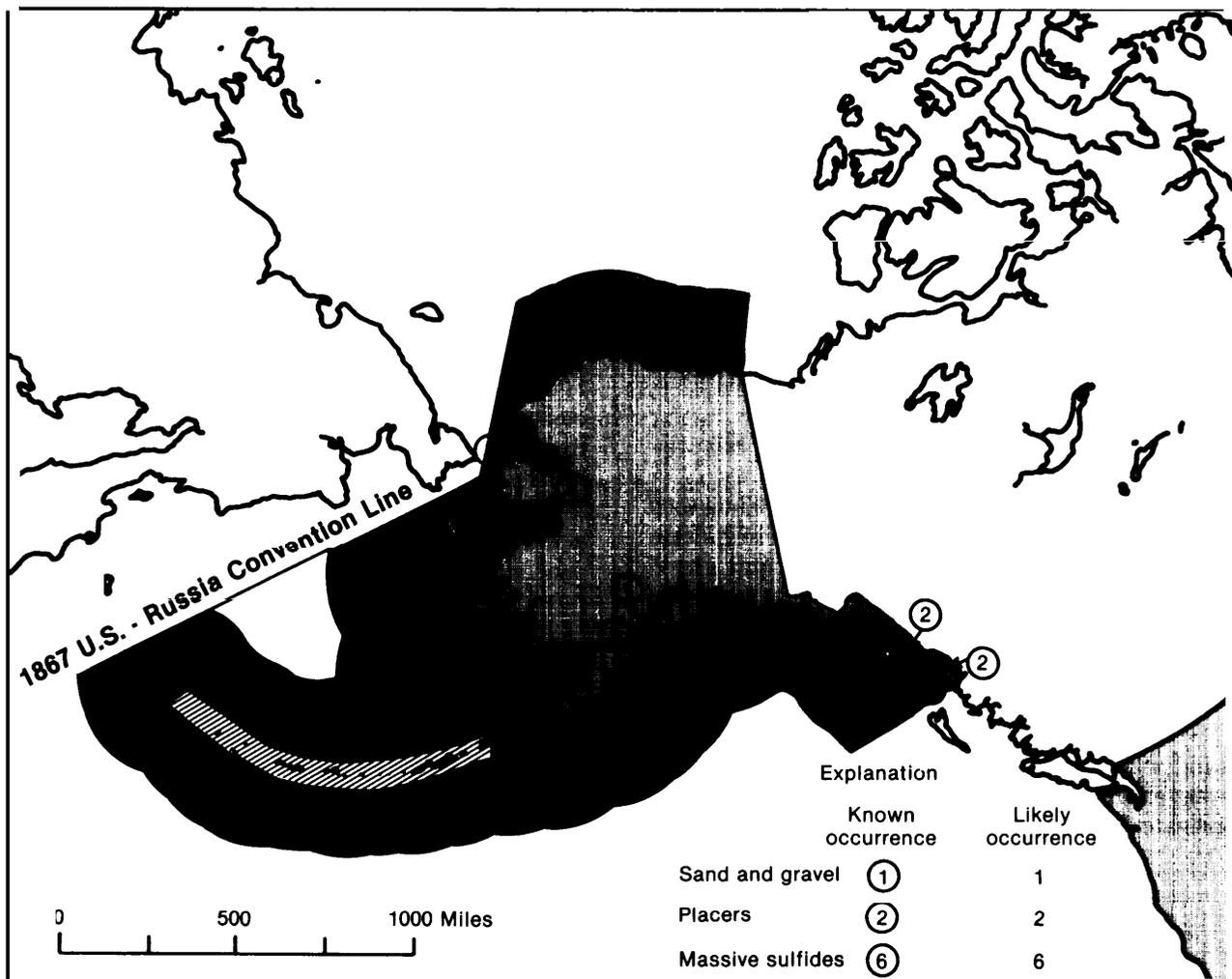
Gold and gravel have been mined from Alaskan waters and the potential exists for locating other offshore placer deposits.
