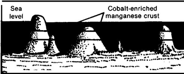
Iron-manganese crusts enriched in cobalt occur on the flanks of volcanic islands and seamounts in geochemically favorable areas of the Pacific. Samples have been recovered for scientific purposes, but equipment for potential commercial evaluation and recovery has not been developed.
