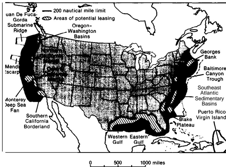
Several basins formed in the EEZ in which great amounts of sediment have accumulated. While of primary interest for their potential to contain hydrocarbons, salt and sulfur are also potentially recoverable from sedimentary basins in the Atlantic and Gulf regions.
