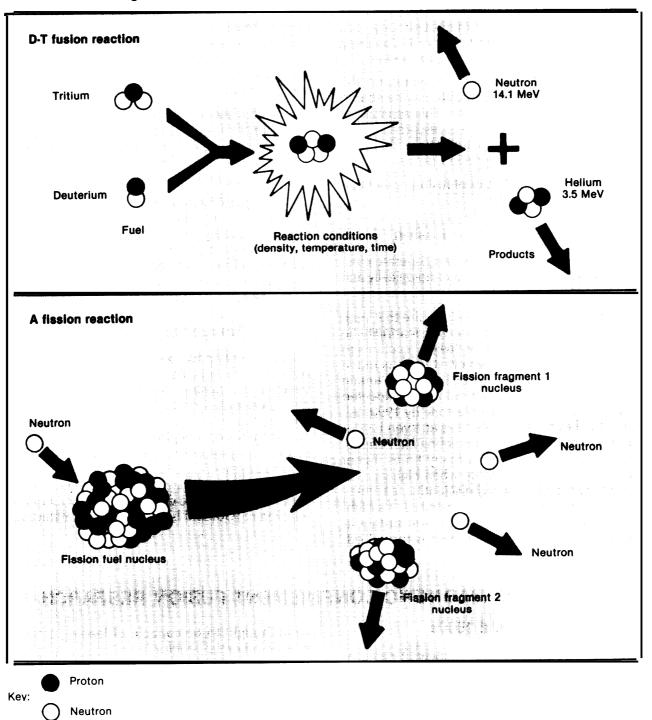
Figure 1-3.—The D-T Fusion Reaction and a Fission Reaction
