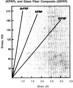
Figure 7-7.—Tensile Stress-Strain Curves for Graphite
