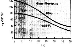
$\acute{o}_{{}_{\rm A}}$  is defined as the amplitude of the cyclicly applied stress.  $^N{\rm F}$  is the number of cycles to failure.
