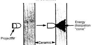
Energy absorption occurs in ceramics and brittle PMCs by spreading local impact energy into a high-volume cone of fractured material.
