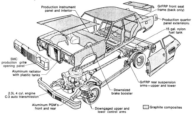
Figure 7-3.— Ford GrFRP Vehicle With the Composite Components Shown
