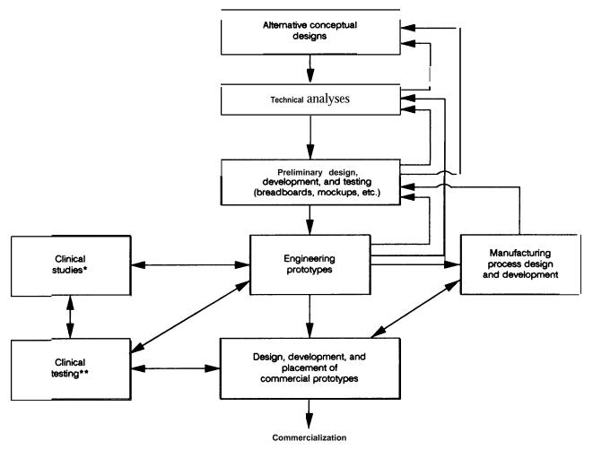
Figure 3.—Development Stages for Magnetic Resonance Imaging (MRI) Systems
