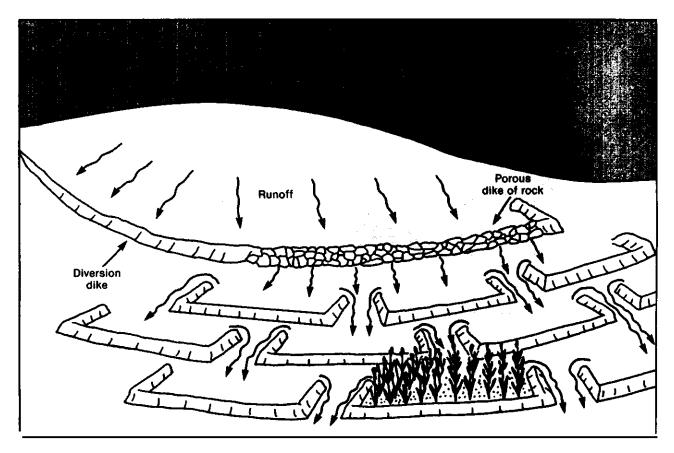
Figure7-1 .— Contoured Microcatchments to Control Soil Erosion and Water Runoff
