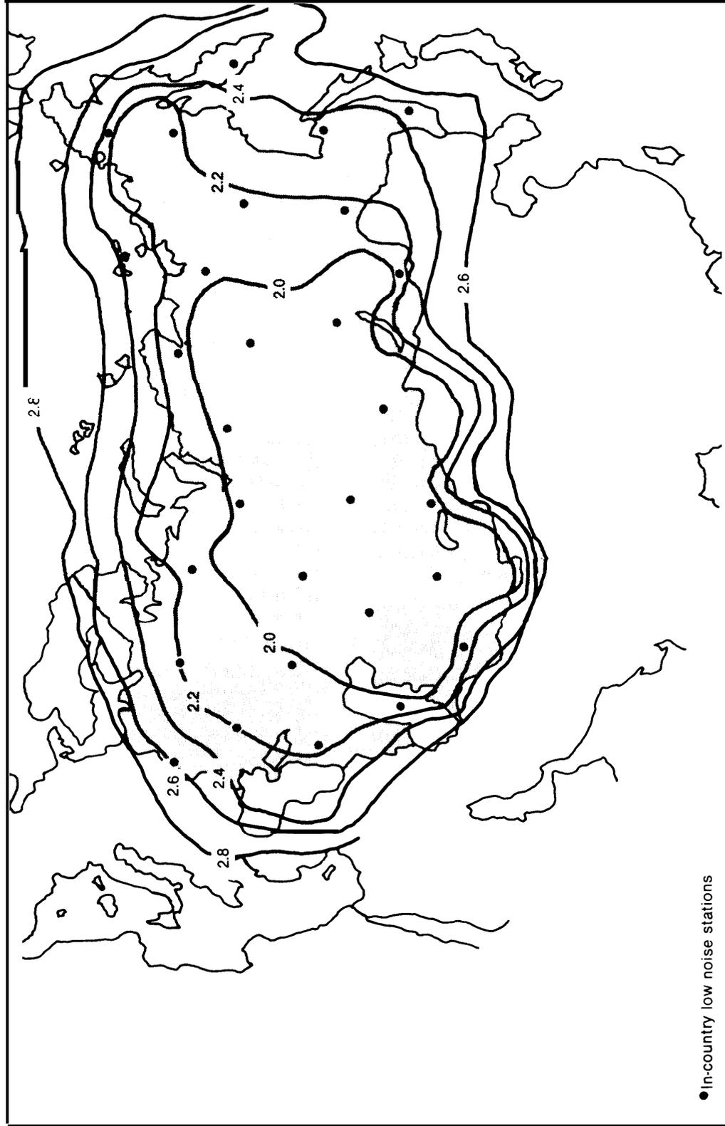
Calculated detection capability (in  $m_b$  units) of an external network plus 30 internal, low-noise arrays.
