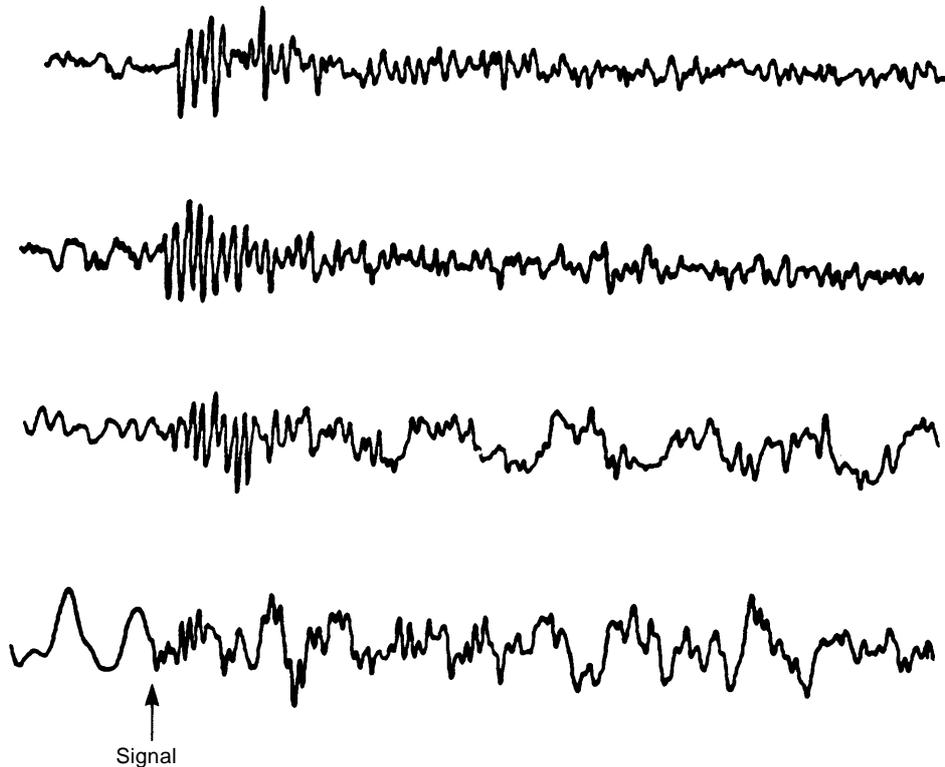
Small seismic signals in the presence of seismic noise at four different stations.
