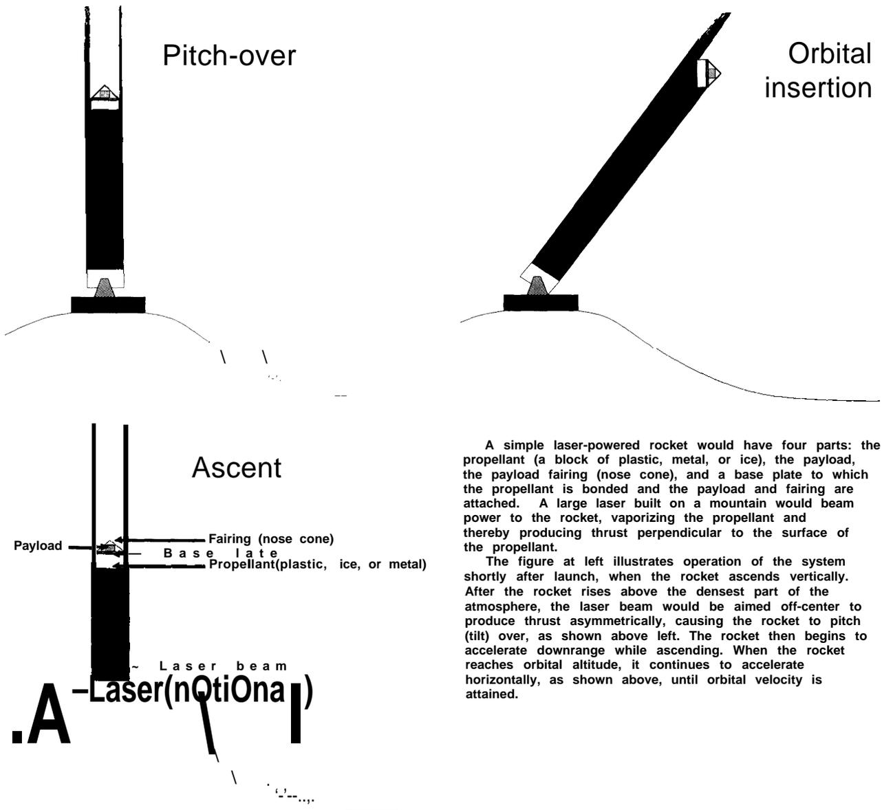
A simple laser-powered rocket would have four parts: the propellant (a block of plastic, metal, or ice), the payload, the payload fairing (nose cone), and a base plate to which the propellant is bonded and the payload and fairing are attached. A large laser built on a mountain would beam power to the rocket, vaporizing the propellant and thereby producing thrust perpendicular to the surface of the propellant.
