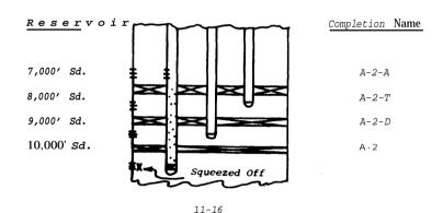
Example No. If 5the A-2 completion in Example No. 4 had. been completed from the 10,000' sand to the 9,000' (where the A-2-D is currently completed), the pletion would still be named A-2-D as both tub strings would be considered one completion fo poses of this Order.
